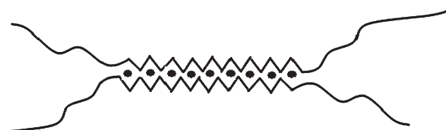
Figure 8 Scheme of the “egg-box” zone ( according to 33 ) formed between the G blocks localized in two adjacent macromolecules. Black dots stand for the calcium ions.
